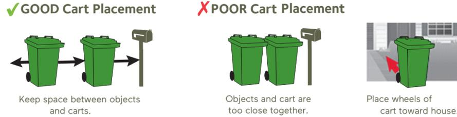
The placement of the cart is very important as the collection vehicle's lifting arm requires clearance of at least 3 feet on both sides of the cart and 12 feet overhead. Carts should be no more than 3 feet away from the roads edge, with the arrow facing the road and the handles facing the house.
